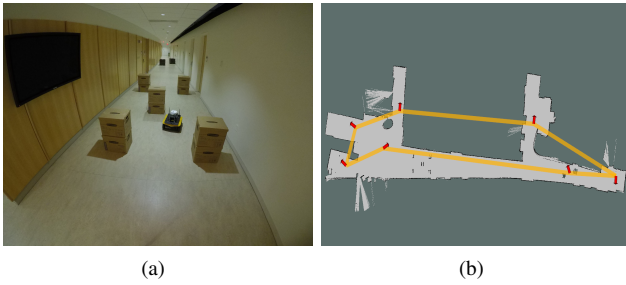
Fig. 12. Basement setup (a) and associated map with watchman tour (b).
